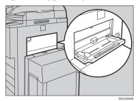
Insert copy paper with the side you want to copy facing up, pusing until you hear the beep, and then align the paper guide to the paper size.
